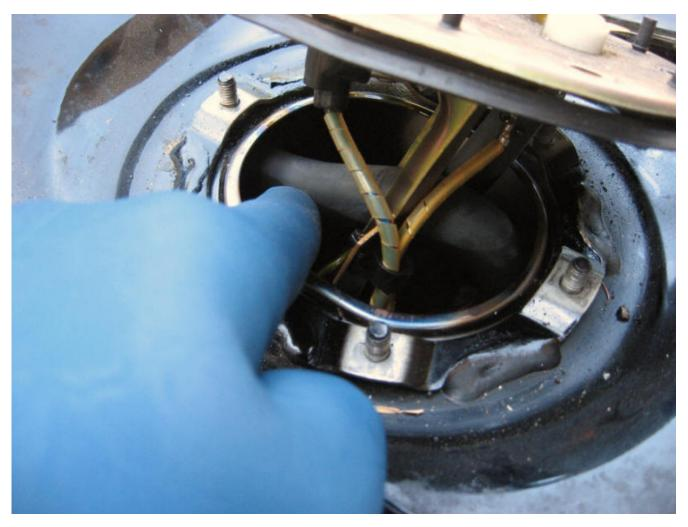
Now you can slowly lift the pump/cover assembly up and out, rotating the top end towards the back of the bike as you lift (see pic).
