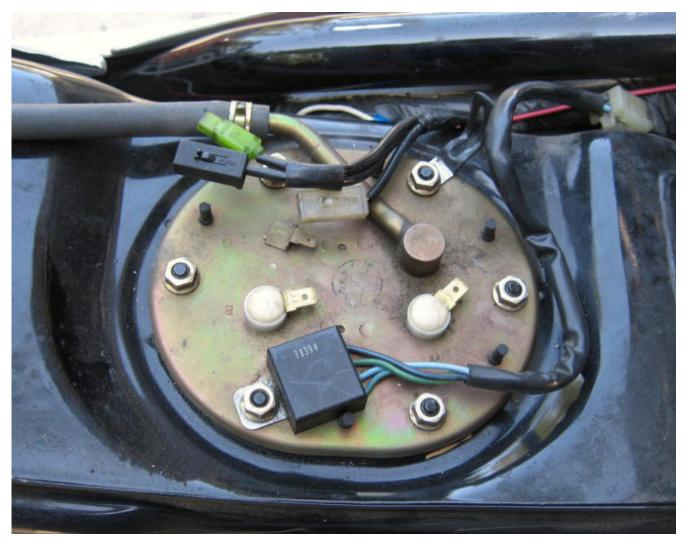
Remove all 6 of the 10mm nuts holding the cover on (don't drop any into the bowels of the bike!) and slowly lift the cover up about 2-3 inches then stop. You'll see a hose leading to the front of the tank (see pic). There is a metal connection right there that you cannot see. Simply pull the hose loose from the connection. There should not be a clamp.
