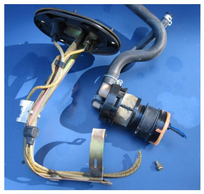
You only need to keep one part from the assembly you just removed. The rubber "donut" bushing that the band clamp goes around. Just roll it off the old plastic pump housing.
