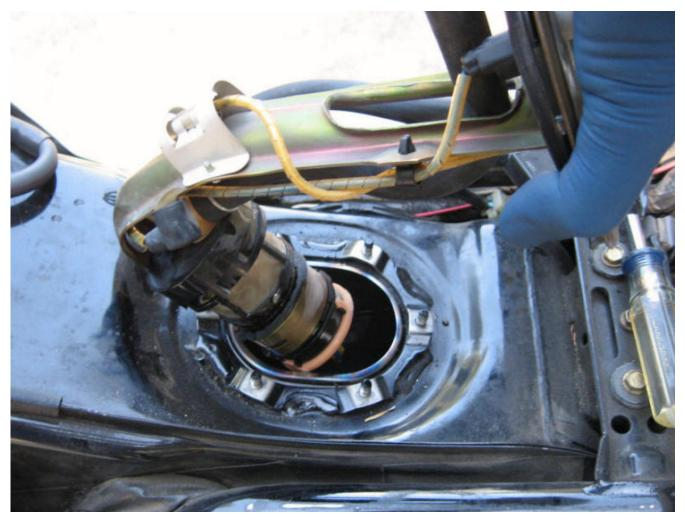
Now cut the 2 wires close to the pump and remove the hose from the fitting on the tank cover. Finally, remove the screw from the band clamp that holds the pump/strainer assembly and remove the assembly as shown (see pic).
